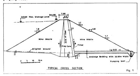
In the first phase the dam wall reached a height of 28 m above the foundation, and a crest length of 415 m. In a second phase, currently being studied, the dam will reach 40 metres above foundation with a crest length of 1200 m. Two small saddle dams were also constructed in the first phase.
